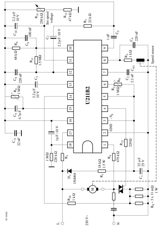
Figure 25. Speed control, automatic retriggering, load limiting, soft-start, tacho control
