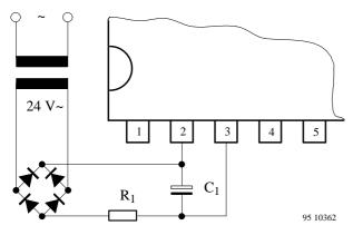
Figure 3. Supply voltage for high current requirements
