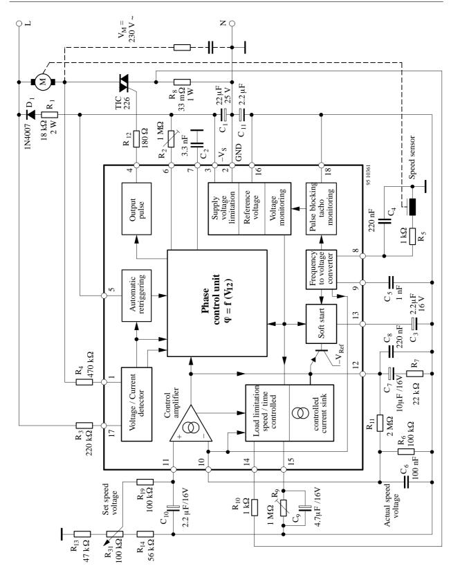
Figure 2. Speed control, automatic retriggering, load limiting, soft start
