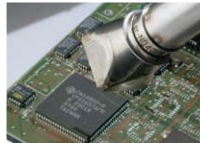
Patented Weller nozzle technology safely removes QFPs, PGAs, and SMT bases.
