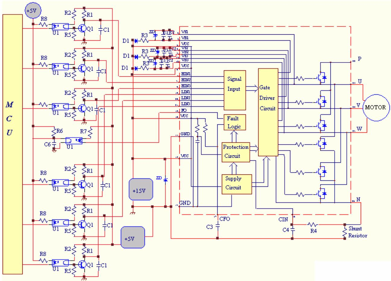
Figure.14 Typical Application Circuit Interface Example with Opto-Coupler
