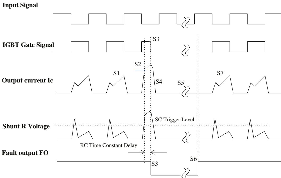
Figure.9 Timing Chart of SC Operation
