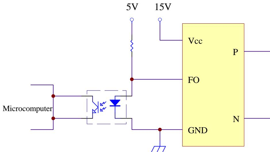
(b) Fault output pin
