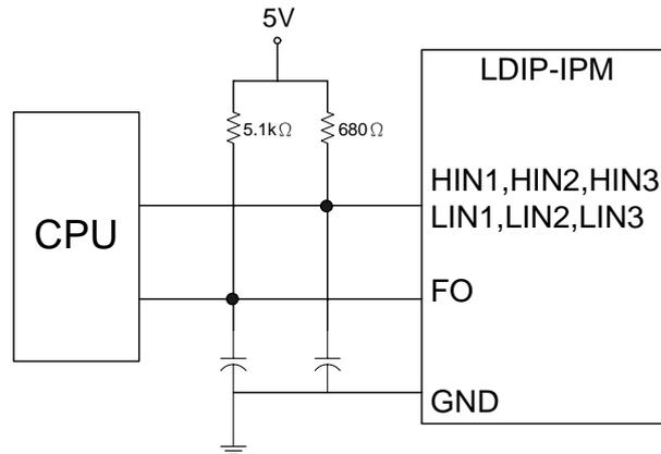
Figure.11 I/O interface Circuit
