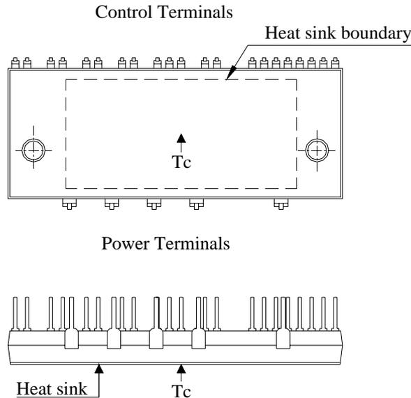
Figure.3  $T_c$  measurement point
