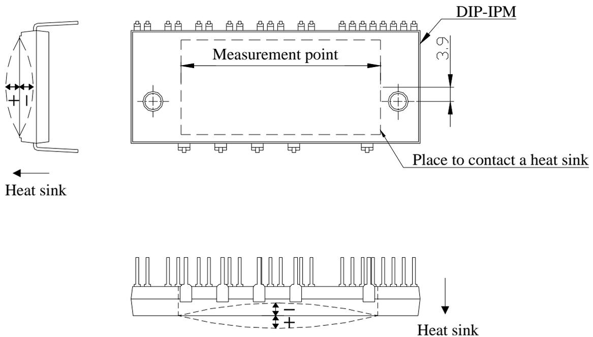
Figure.6 Measurement point of heat-sink flatness
