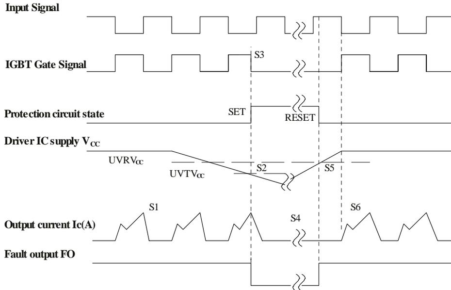
Figure.10 Timing Chart of Under-Voltage Operation
