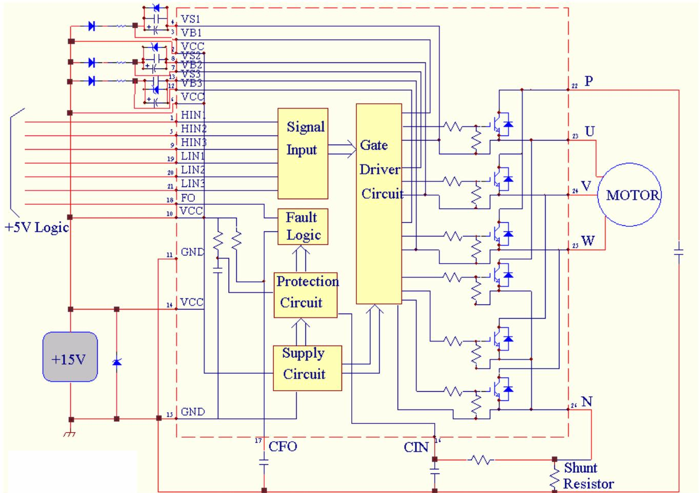
Figure. 2 LDIP-IPM Internal Block Diagram
