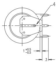
Note: 1)No welding onto the groove 2)For typical PCB—application we recommend to use VARTA—Mempac batteries. 3)\* For reference only
